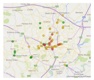
Air quality across Coventry's diffusion tube sites in 2019 (above) and 2020 (below), where green sites have annual mean concentration of nitrogen dioxide of less than 30 microgram per cubic metre ( $\mu$ g/m3); amber sites between 30-39  $\mu$ g/m3; and red sites with 40  $\mu$ g/m3 or above. Note that 2020 figures are likely to be an anomaly as lockdowns resulted in a marked reduction in traffic.
