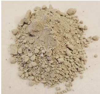
Chalky soil from soil investigation
