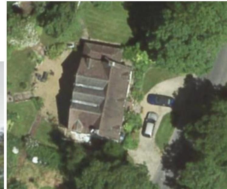
The extensions and additions added over the life of this building have made for an interesting and complex multiple pitched roof form which isn't obvious from the road.
