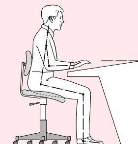
Figure 9 Tilting seat - shown here with sloping worktop - to improve comfort and reach
