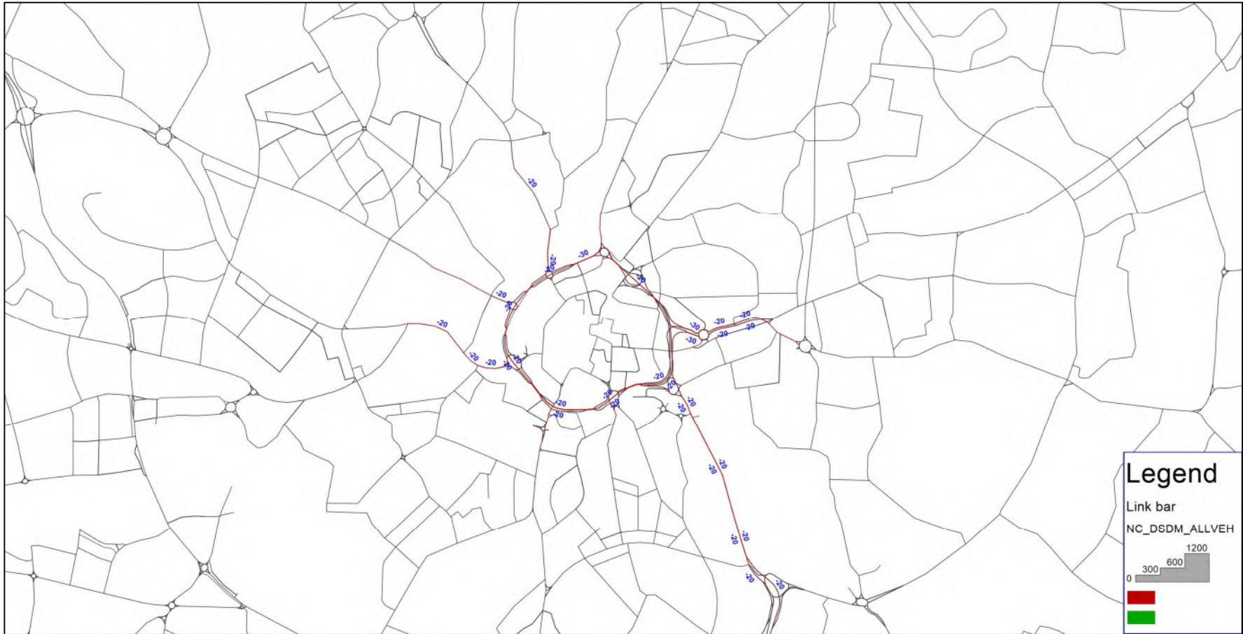
Figure 41: AM peak Flow Differences between 2031 DS 2b and 2031 DM Scenario (Non- Compliant vehicles) City Centre
