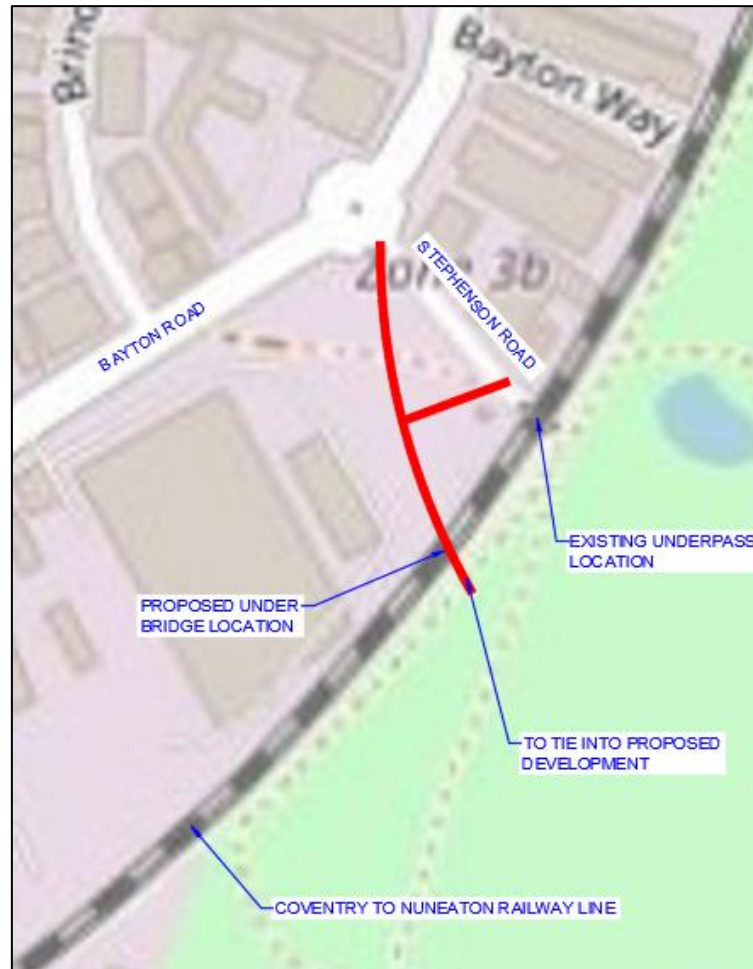
Figure 6-5 - Proposed off-line alignment - under the railway
