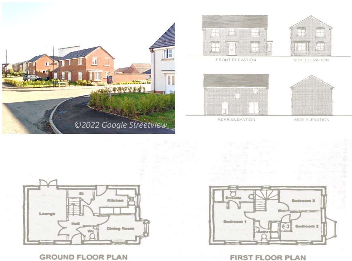
Figure 24: sketch diagram to show floorplan and elevation for a dual aspect dwelling
