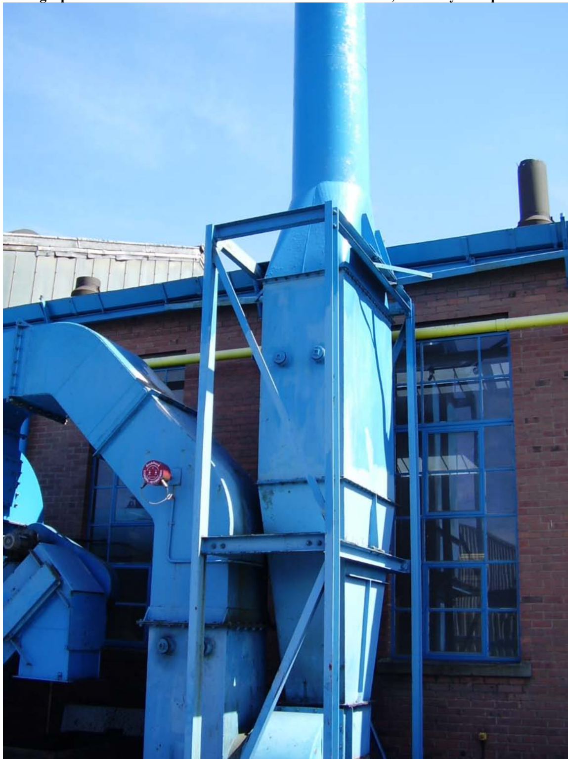
Photograph of PMA1 Main Scrubber Stack at Atritor Limited, Coventry in September 2005
