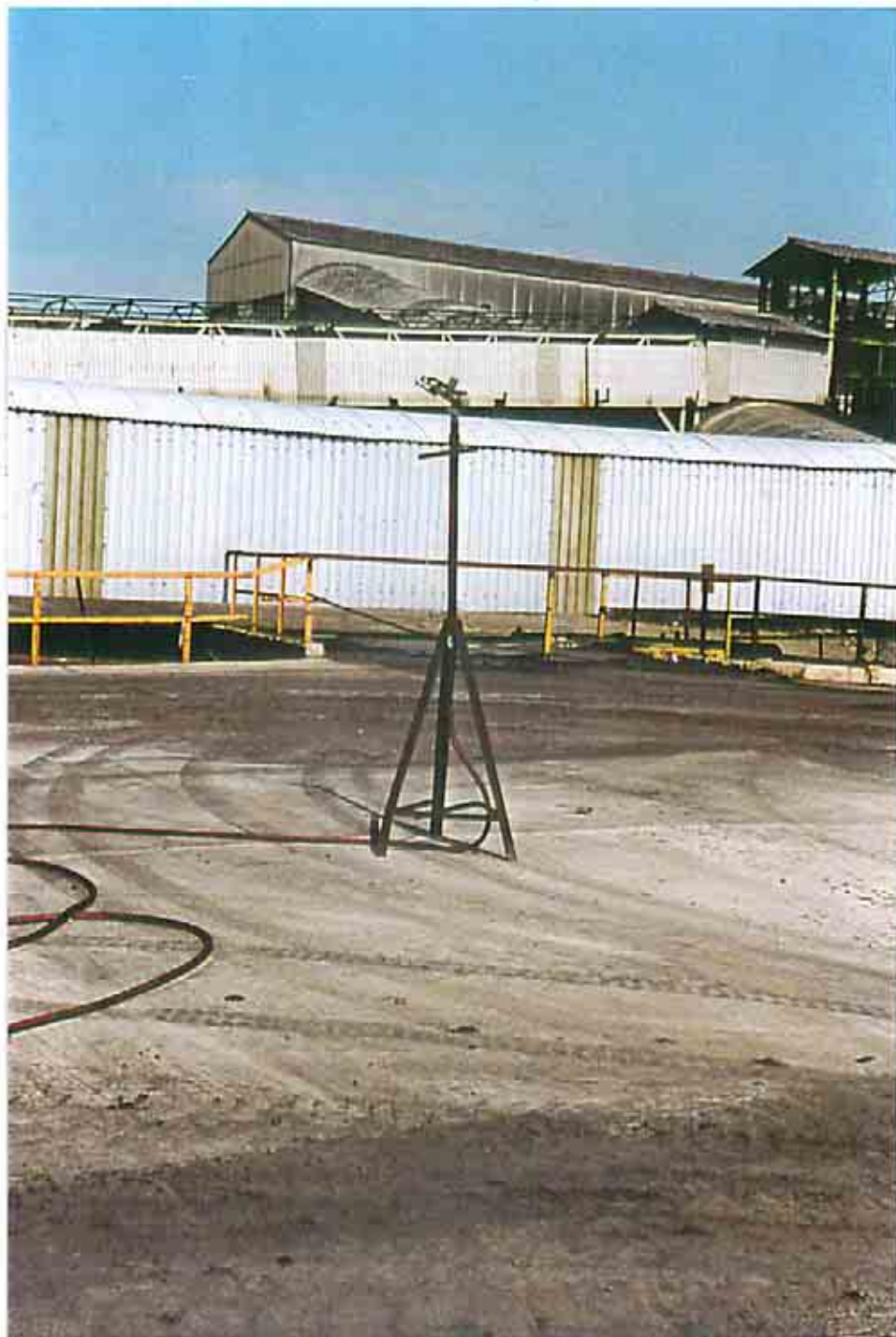
Mobile Spray Used for suppressing dust on open stocked product.
